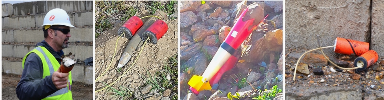
From Left to Right: Former ATF agent Steve Beggs providing practical demonstration on UXO removal; Howitzer 105-mm round UXO removal set-up; Unexploded avalauncher charge; Unexploded booster hand charges.
